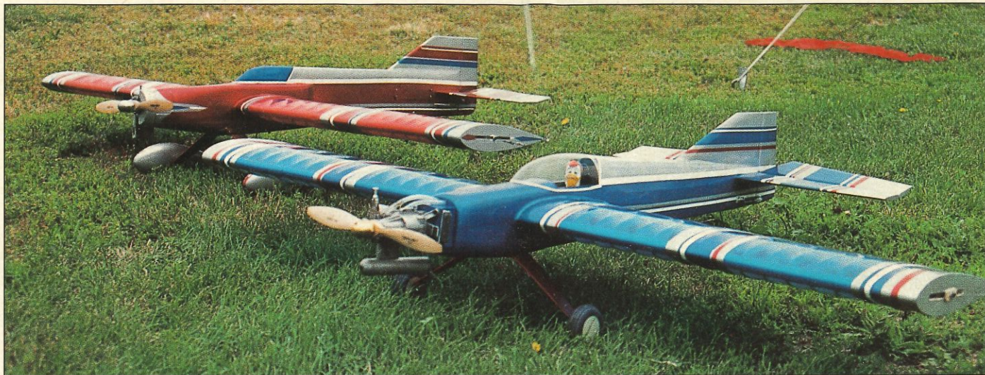
This photo illustrates the Twister Sister's ancestry. In the background is a Twister II, otherwise known as a "Fancherized" Twister; it's a Sig Twister kit with modifications as outlined by CL Stunt legend Ted Fancher. In the foreground is the author's prototype Twister Sister, built per the plans presented here. Power is a K&B .28 Sportster with a Davis diesel conversion head.
