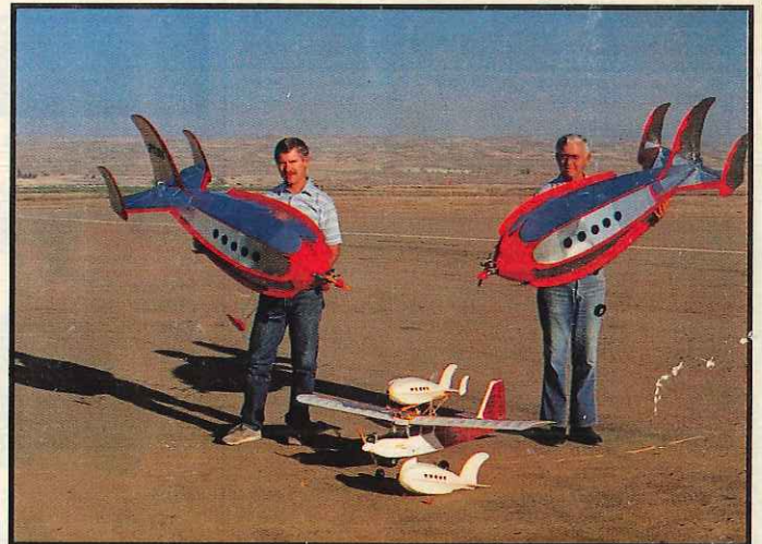
Designer Skip, with dad, Gordon (right), portray actual size of model. The two white "Cubs" are styrofoam test models. One is mounted on "Piggy Back" rig on Sig Kadet, used for higher altitude "glide" tests.
