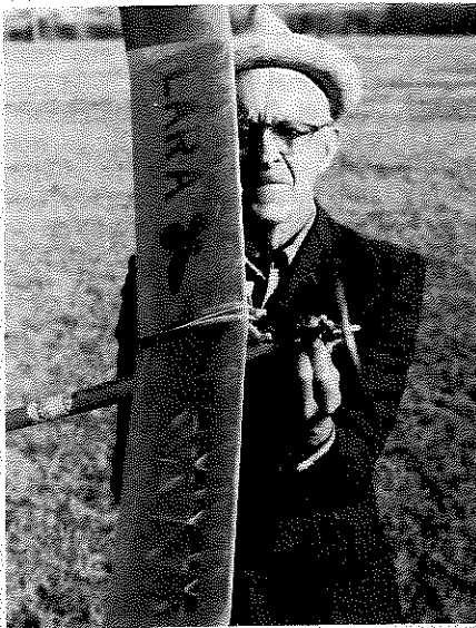
LARA's designer, Reid Hull, needles the Cox TD prior to a test flight.
