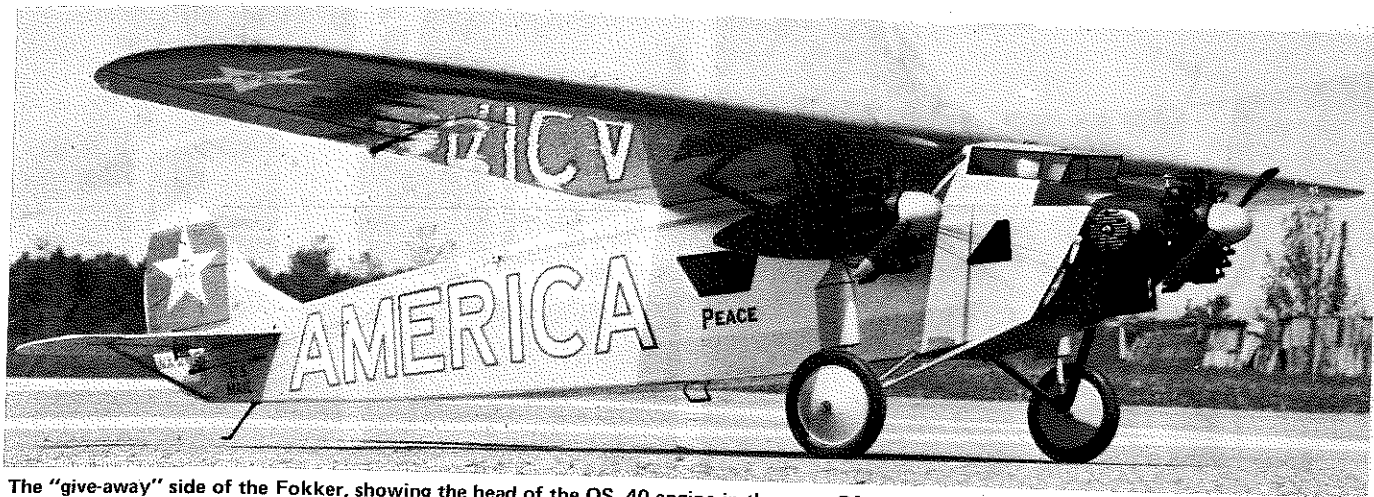
The "give-away" side of the Fokker, showing the head of the OS .40 engine in the nose. Of course, the outboard engines are dummies, with the scale-like props being allowed to free-wheel. High pitch on these reduces drag. Note external control cables (scale only).
