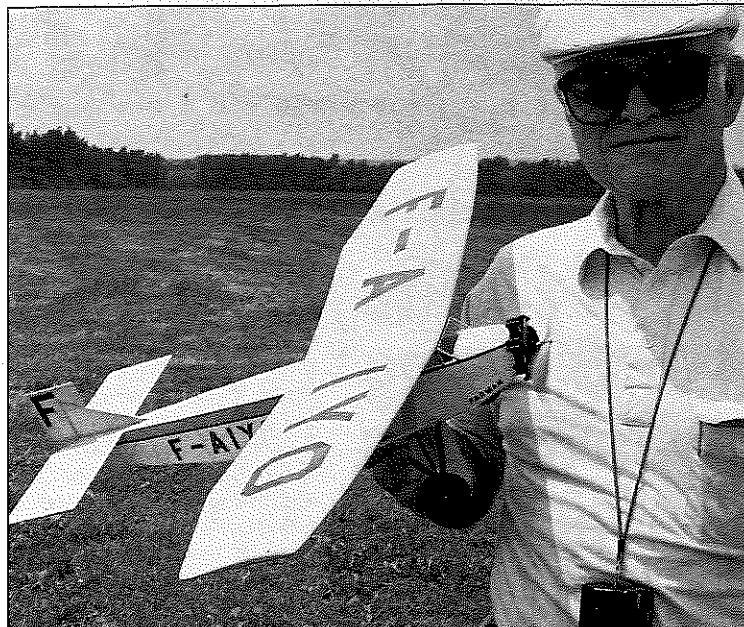
The author takes a break with his 1920s French monoplane. The brightly colored 28-3/4 inch span model is finished in white and yellow Floquil paint with black lettering; details for a silver-and-white aircraft with red lettering are included on the plan. Power is a HiLine "Mini 6" electric power system.
