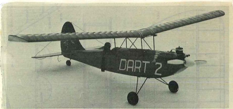
The completed Dart 2 ready for test flights. This one is powered with a Thunder-Tiger .25, but the Dart 2 will fly very nicely on a .19. (That's snow under those tires, not concrete!)
