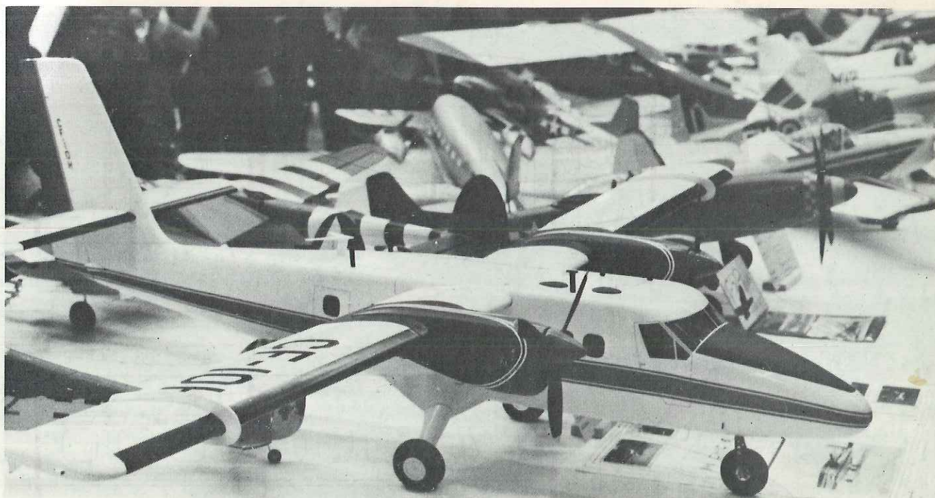
Twin Otter model built from these plans by Dave Allen, Ontario Canada, and shown at the 1974 Toledo Trade Show. Long, skinny wing is evident in this photo, also wing fences, which are not on the Golden West aircraft seen at Orange County.
