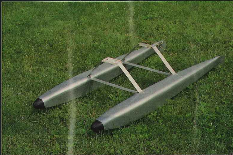
The floats were designed specifically for the Osprey, with Sullivan cable linkage to the water rudders.
