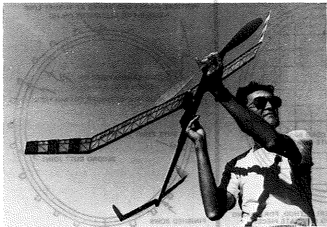
Author's prop is carved from Pacific Cedar Pine and uses special ARA-D airfoil for extra thrust, thus allowing fewer strands of rubber for a long 50-second power run.
