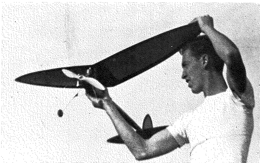
Here's Tom (a little younger, but not much thinner than he is today, the lucky bum!), holding his all sheet balsa gas model in launching attitude. Span is 48 inches.
