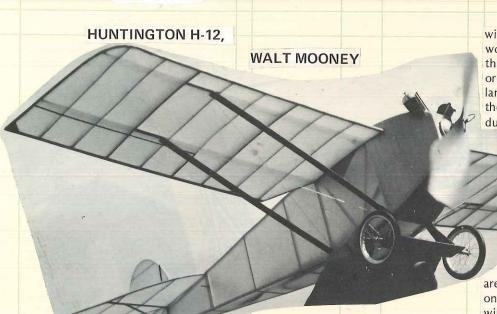
This is a model of one of the first homebuilt airplanes in the U.S.A. Not that all the first airplanes weren't really built at home, but this was designed after WWI and was actually intended to be built by amateurs. It used a two cylinder "V" type engine, undoubtedly out of a motorcycle. It was truly an attempt to obtain an airplane for a minimum first cost.
