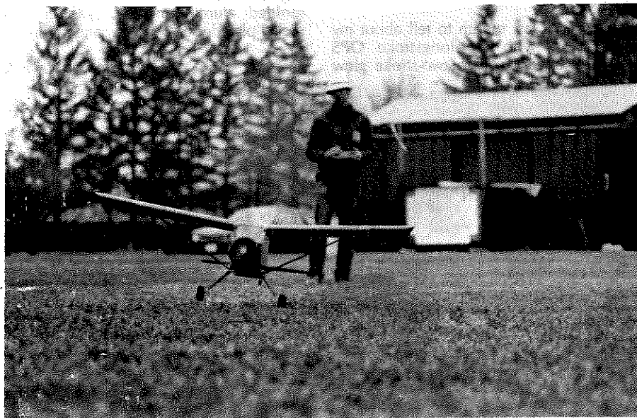
The author's Beaver , eagerly heading for the cameraman, comes in at 48 ounces. Power is from a Leisure gear drive 05 system, with a six-cell 1200 mah Sanyo battery pack.
