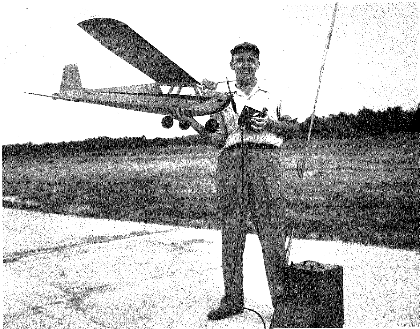
A happy Walt Good after his 1952 R/C duration record flight of 40 minutes, 28 seconds, at Andrews Air Force Base, near Washington, D.C. The model is his 6-foot Rudder Bug, with a Forster .29 ignition engine. Transmitter control box is in his left hand. Radio is described in text.
