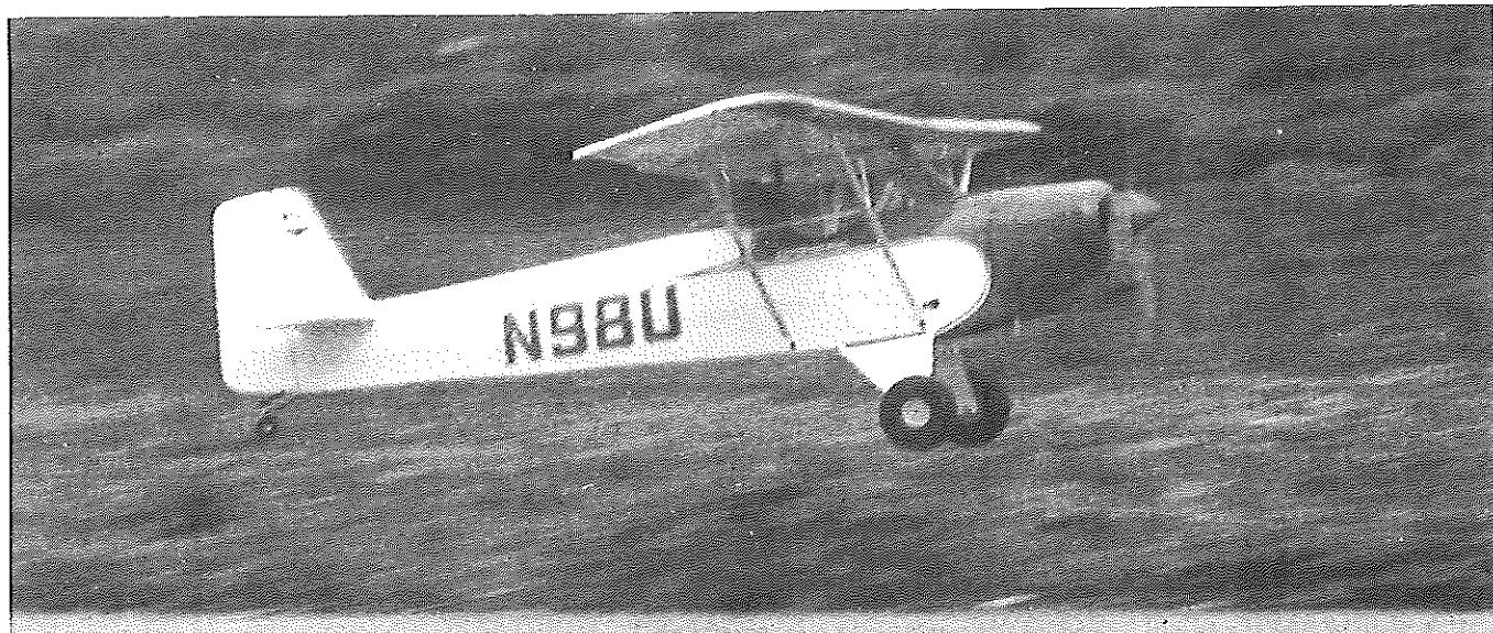
The moment of truth, at liftoff of the model's first flight. Aside from a slight left yaw, corrected with rudder trim, and later with push rod adjustment, no further trimming was necessary. The Du-Bro reduction drive unit functioned perfectly. Engine was hand-propped for starting.
