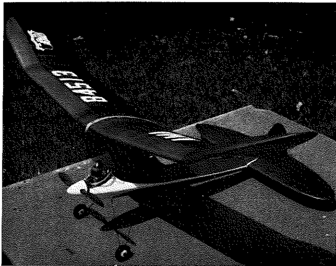
15. This snappy looking Swoose was built by Maurey Fine. Orange and white color scheme, and O&R .29 front rotary valve motor.
