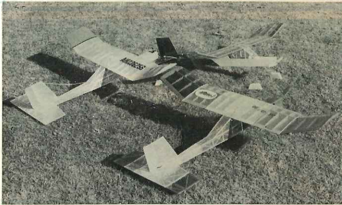
Big Bird the E.T. is a scaled up and modified Peck-Polymers Prairie Bird rubber powered model. Really shines as an electric trainer.
