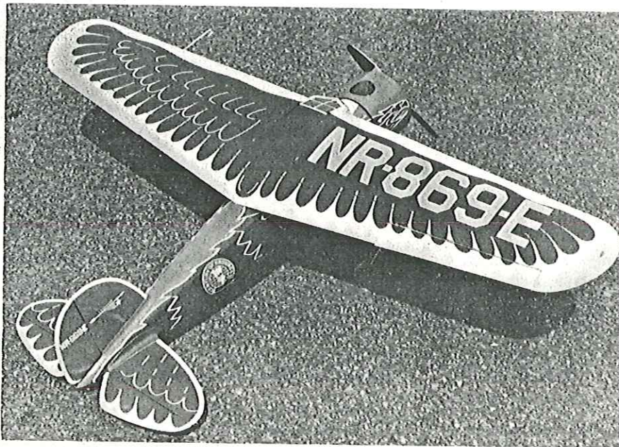
Only one application of masking tape required for three-color paint scheme. Start with white base. Note raised fairing lines. Small lettering is rub-on type.
