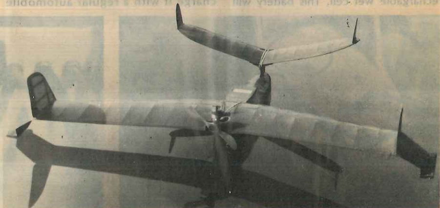
You'd have to have quite an imagination to dream up a stranger looking model than the Pelican. Model uses an old Taipan .09 diesel, but a Tee Dee .049 would probably work well also.
