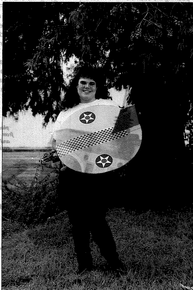
■ RIGHT: Miss Sunny Chevez displays the completed O.S. .25-powered Floppy Disc shown being assembled—in about an hour—in the following photos. Advantages of the corrugated polypropylene material are that it's cheap, is readily available, comes in a myriad of colors (including fluorescents), is easily worked, assembles quickly with CA glue, is completely fuelproof, and is incredibly tough. For "quick and dirty" model construction, what more could you ask? ■ ABOVE: Floppy Discs have also been flown with electric power, all the way up to Astro 15 Cobalts—this particular model uses an Air Supply motor with a Master Airscrew prop and gearbox. Open section of the fuselage top just in front of the wing provides cooling air to the batteries.
