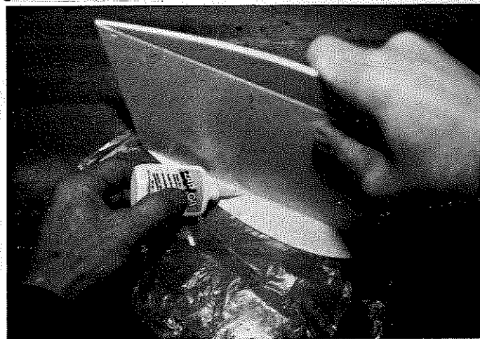
Aerolite (1/16) construction of float: score inside of bend, fold 90°, Zap inside of bend. Simple, quick, neat!
