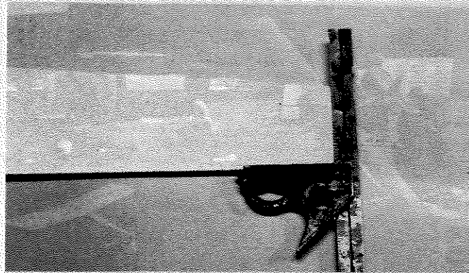
Also square off tip, cutting it at 90 degrees to the trailing edge.
