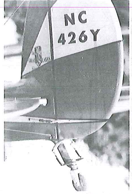
Steerable tail wheel is legal modification. Steering arms linked to rudder with springs.
