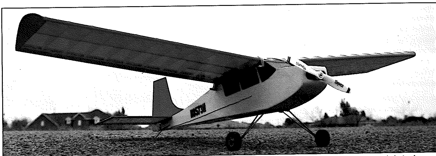
From any angle, the Electric Scout is a fine looking model. Author's prototype is covered with a combination of MonoKote and Ultracote. Keep it as light as you can for best performance.
