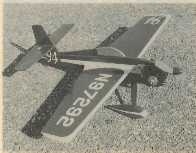
The senior O'Reilly's Little Mike. Model uses the sheet aluminum landing gear and engine mount shown on the plans.
