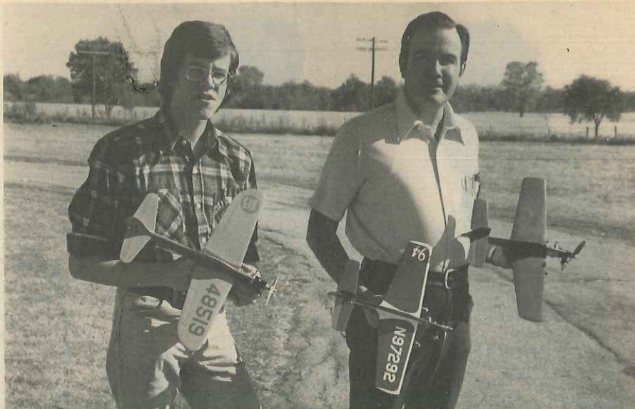
The authors with their 1/2A racers, all powered by Cox Black Widows. Little Mike in center was built when incompatible paints on first Little Mike (right) ruined the finish.
