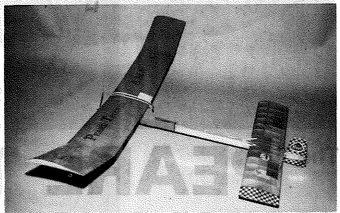
Three different views of the "Pearl Trucker". It is a cross between Bill Chenault's "Pearl" series and Sal Taibi's "Starduster". Designed for flying at Denver's mile high altitude, it climbs like a rocket at normal levels. Thick stab (9%) eliminates need for auto-surfaces.
