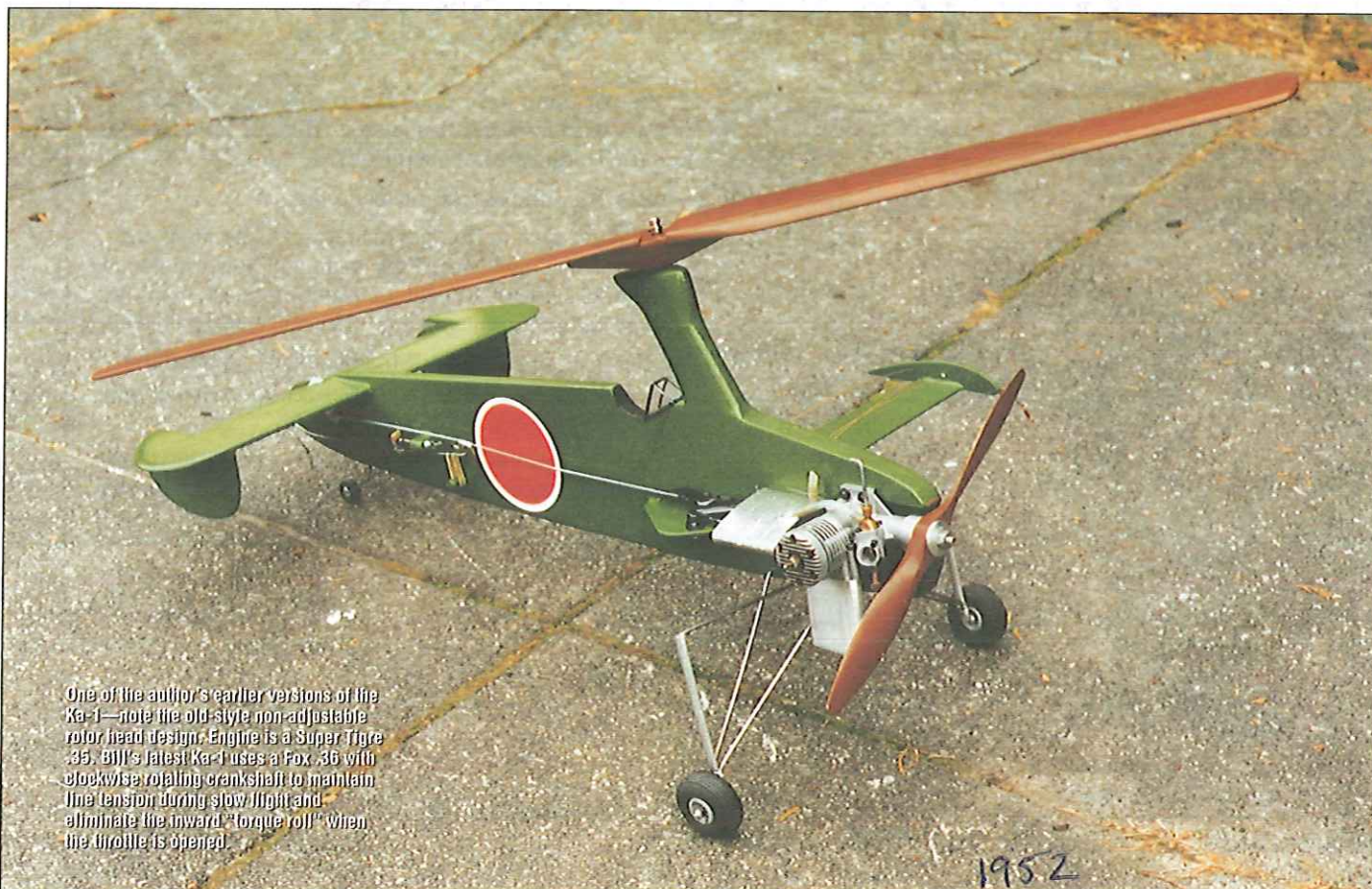
In fully developed slow flight the Ka-1 has been clocked as slow as 10 mph; here the rotor is operating at about +38 degrees from horizontal. Best of all, an autogyro can fly like this naturally, without resorting to line sliders or any of the other fancy tricks the fixed-wing guys have to use to achieve the same thing.
