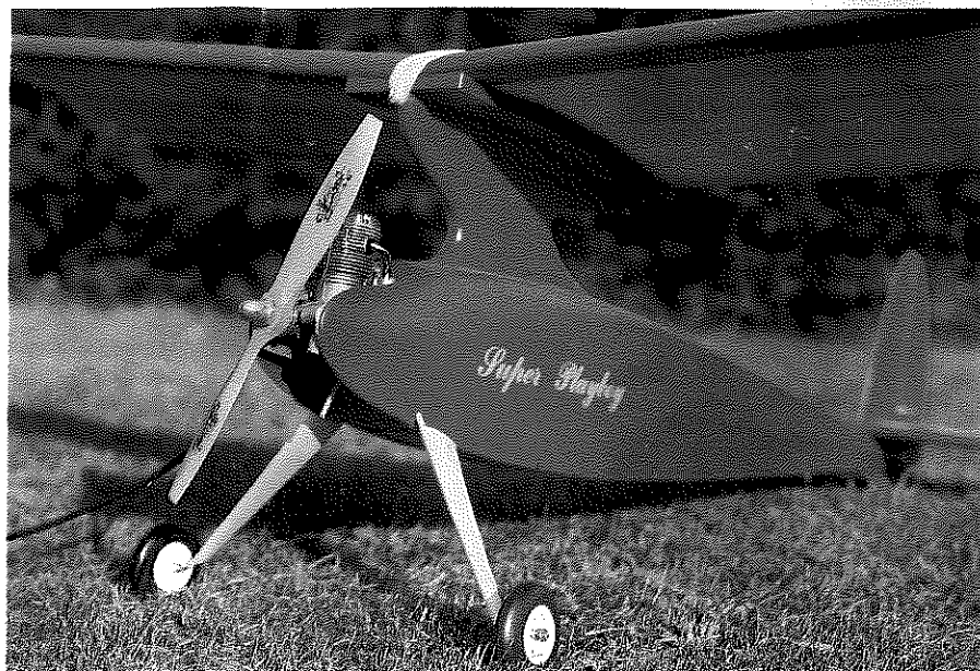
With a wingspan of more than nine feet, the nine-pound weight of the Super Playboy was relatively inconsequential. With care, it can be built much lighter without sacrificing strength.
