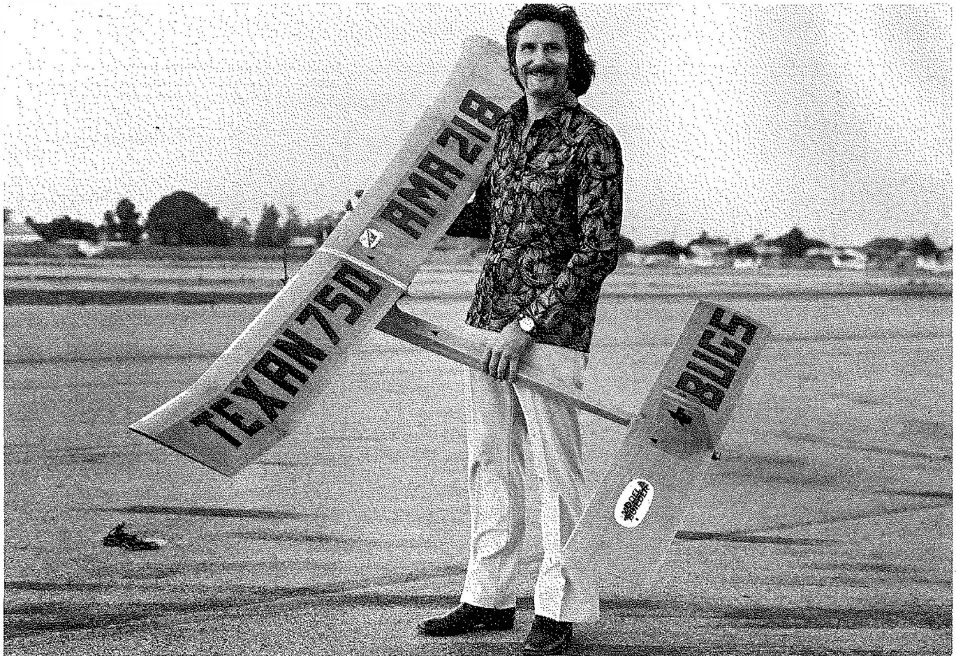
The author, Jim Scarborough, Dist. X Associate Vice President, with his Texan 750. Modifications to the original design include reduced stab area, longer tail moment, and higher pylon.
