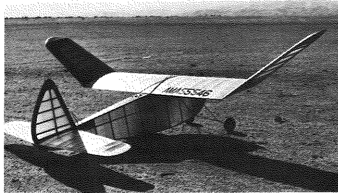
What could be a better combination? Ultra simple to build, and ultra stable to fly. Note DT. Fin goes into slot when popped up.
