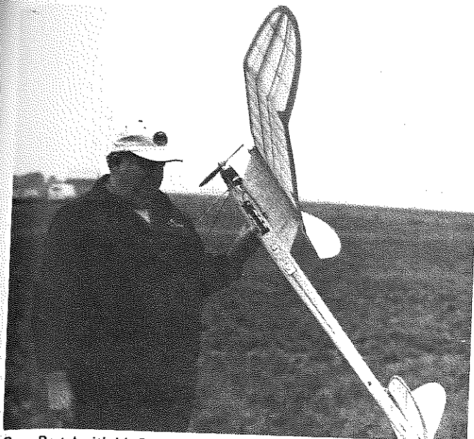
Gene Bartel with his Satellite 788 GLH, powered by a large Astro Flight electric motor. Power system added 20 ounces to total weight.
