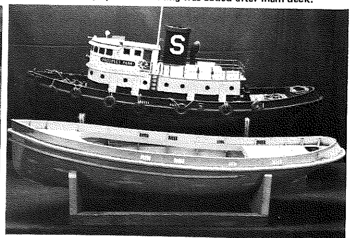
Several hulls were built from plans, assuring accuracy of parts fit. Fender strips have been added to outside of hull.
