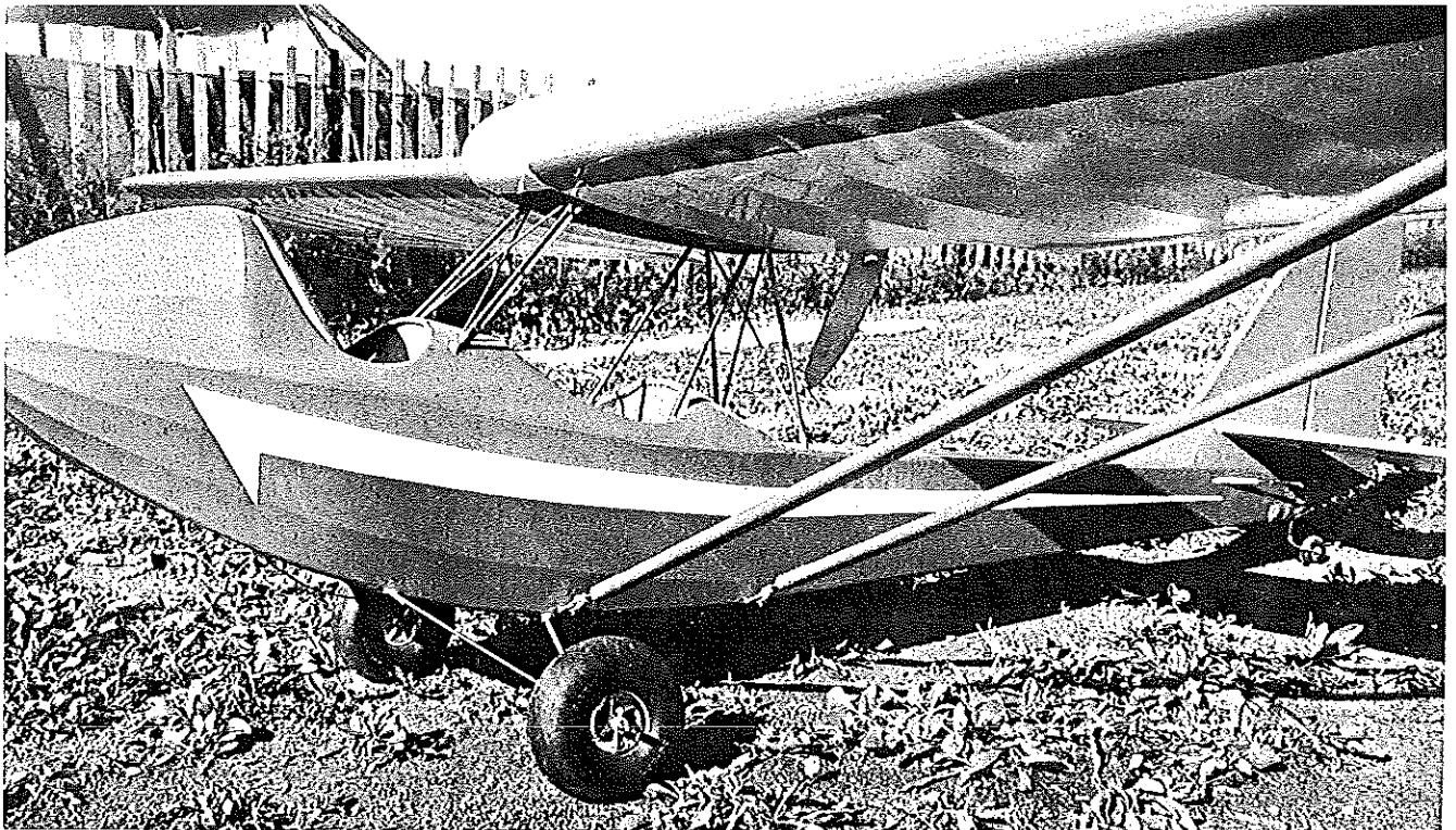
Close up shot reveals an extra strut added on by Ralph Fidance to beef up the landing gear for rough field landings. Ain't that a little cupcake?
