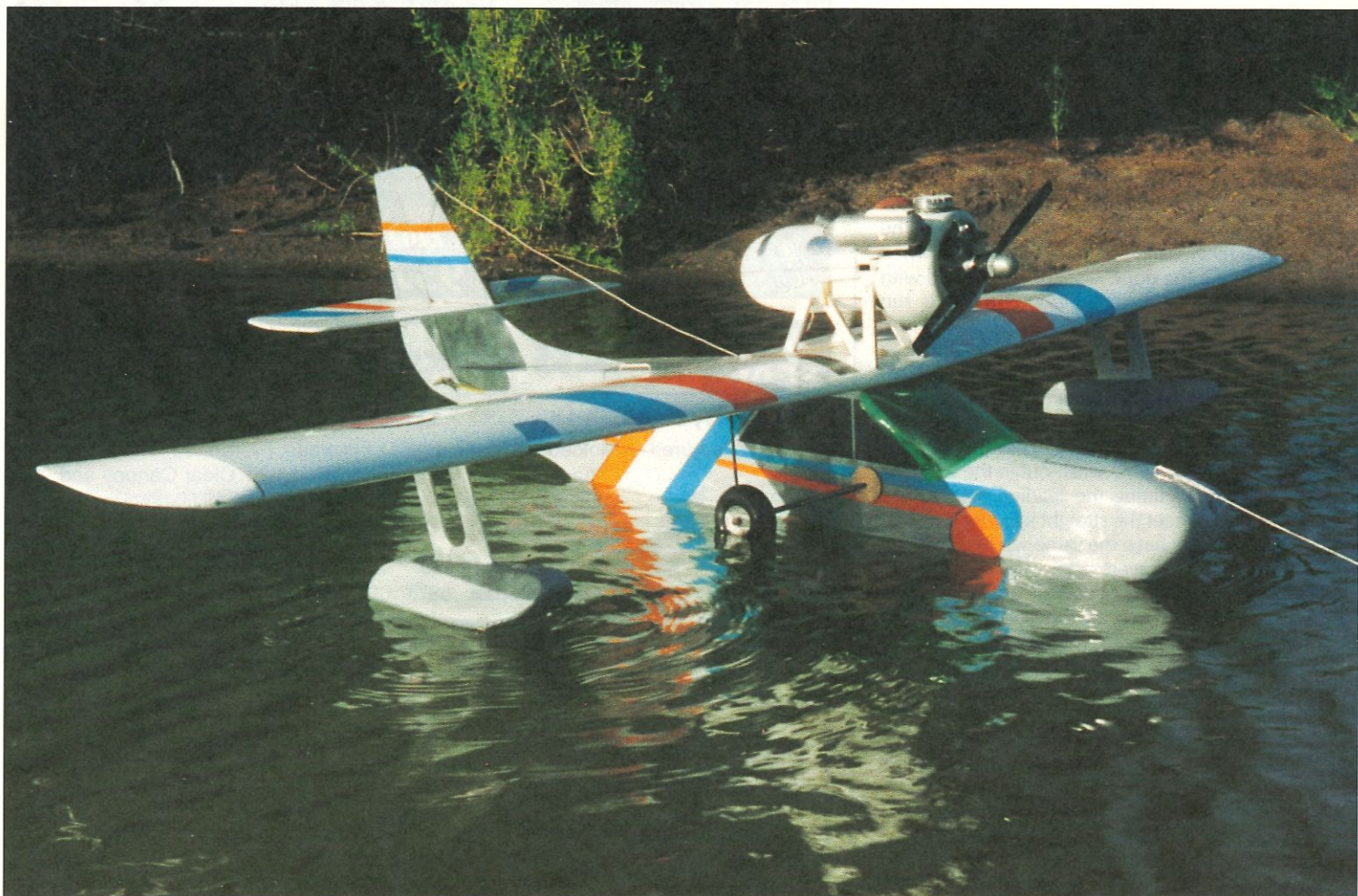
Ain't she pretty? Model's generic design lends itself to all sorts of attractive color schemes, from WWII military to contemporary civilian as seen here. With the exception of the painted engine nacelle, the prototype Wet 'r Dry was covered entirely with Top Flite Super MonoKote, the author's preferred material for all of his EEE-Z-FLI projects.
