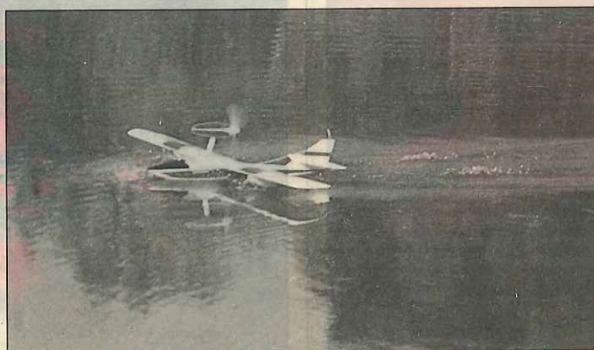
Above: The Seawind seen here with the optional two-wheel landing gear detailed on the plan. Note also that while the author's model sports a clear canopy, the plans show a fully-sheeted, built-up balsa structure.
