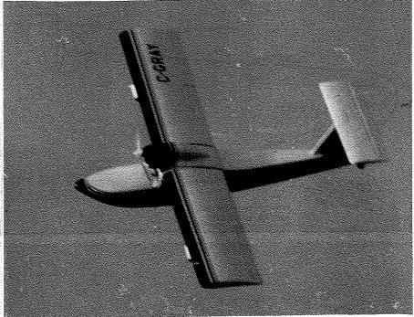
• The Seasport II was designed as a result of a burning desire I had to have a large flying boat for sport flying at the local water flying site. The design criteria were: something with a large wing area so it would float along slowly as it flew, a wide hull so that it would ride up on the water nicely and to utilize a Supertigre .60 Bluehead engine I had which always had been a
