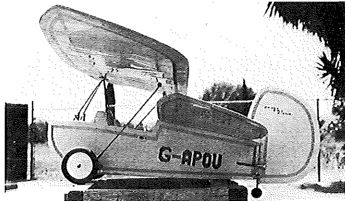
Side view of the Flooing Fly . . . er, Fleeing Floo . . . you know! Elevator pushrod clearly seen here. Darned unusual aircraft!
