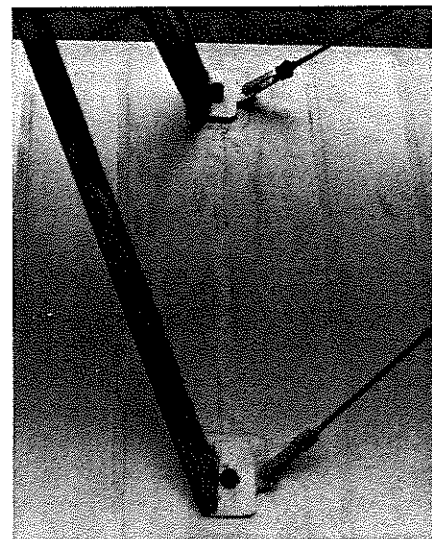
Close-up view of landing wire fittings. Alternate method of attaching struts to fittings shown.
