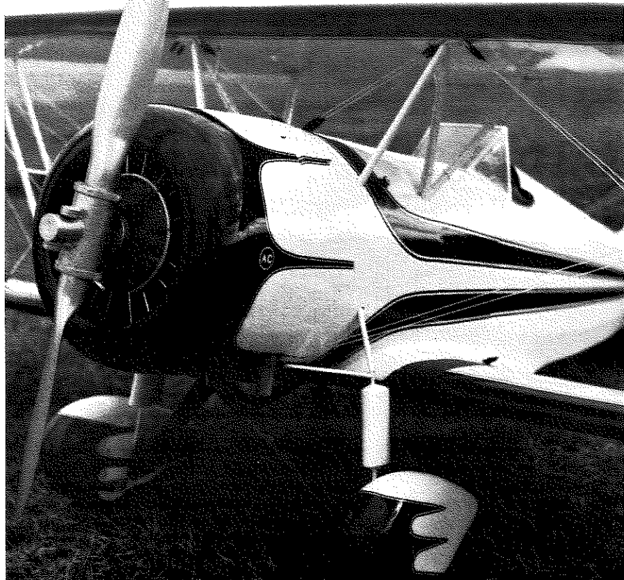
Larry certainly knows how to put on a nice finish! Fiberglass cowl and wheel parts are available from him, direct. See text. Dummy engine from Air Design.
