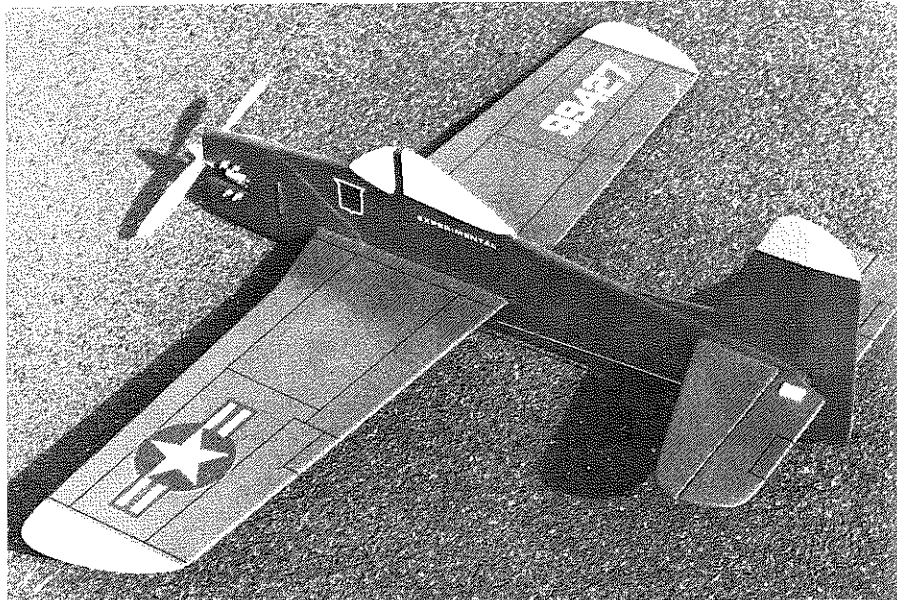
All sheet construction, very little shaping. Great for a beginning scratch builder.
