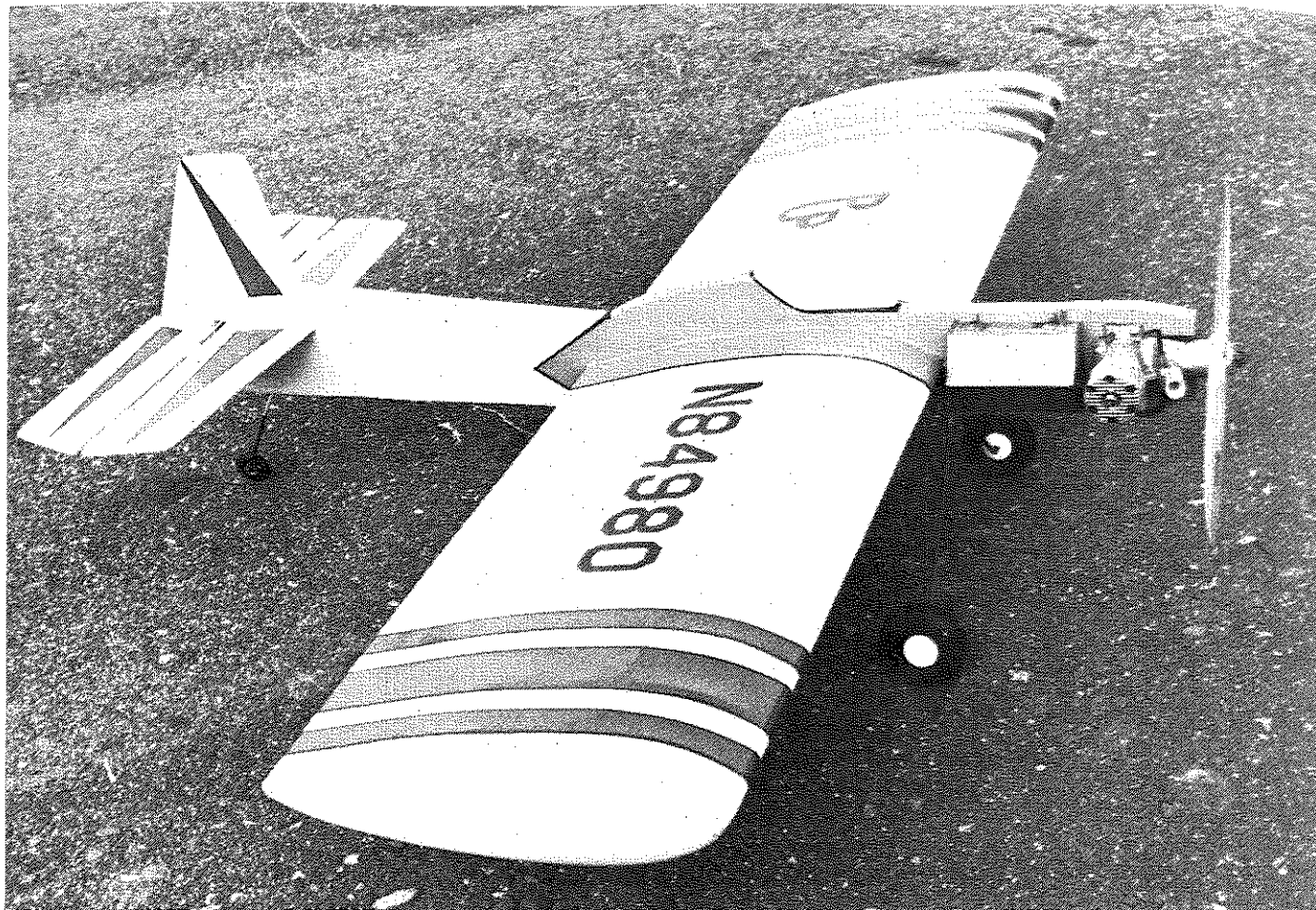
The Pup proves that it's not necessary for a simple profile stunt model to look dumb. Ship is designed for .29 to .36 engines.
