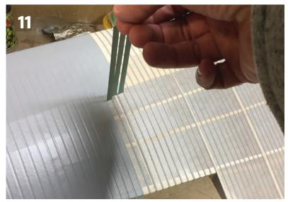
covering with pencil. After wiping down the wing with a clean cloth to remove dust and fibers, the tape was applied from root to tip by eye. The placement of the low-tack tape was easy to adjust. After only two episodes of *Game of Thrones*, the wing was done.
