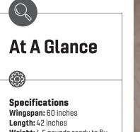
Length: 42 inches Weight: 4.5 pounds ready to fly Power system: 650 Kv brushless motor; 60-amp ESC; 4S 3,700 mAh LiPo battery
