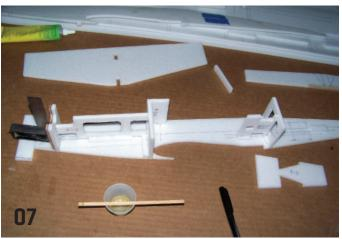
Now is a good time to cut the slots for the CA hinges. Mark the centerline on the wing and the control surfaces. Use four small hinges for each aileron, three or four for the rudder, and six for the elevator. Only apply foam-safe CA where the hinge enters the airframe. Install the hinges in the wing, the horizontal stabilizer, and vertical fin if a rudder is used. Use CA accelerator to speed up the process.
