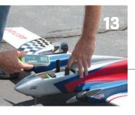
In using pairs of both 3,700 mAh and 4,100 mAh batteries, another solution became evident. When I used the lighter batteries, the rolls improved, but spin entry was not as good. The 4,100 mAh batteries give consistently good spin entry and exit, but the rolls
