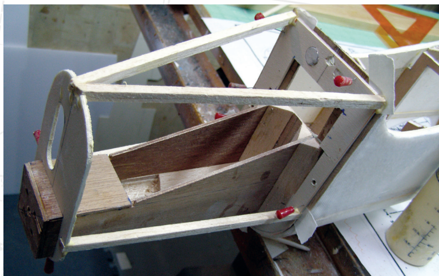
Depending on the length of the electric motor, the length of the box must be adjusted so that the propeller clears the cowl.
