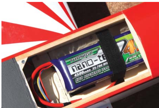
The battery hatch has been removed, showing the 4S 4,500 mAh 35C LiPo battery with a Velcro strap. This size battery is good for 8 to 10 minutes of spirited flying. It can be moved fore and aft as needed to attain the correct balance. The hatch is held down using magnets and a dowel pin.
