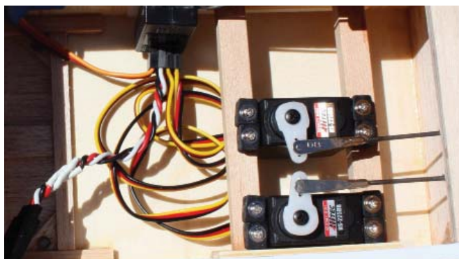
The radio installation shows the rudder and elevator servos on spruce rails. The receiver is held in place to the left fuselage side with Velcro, and a soda straw is installed as an antenna holder.
