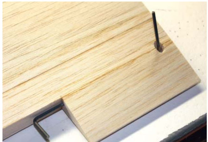
The inboard TE stock with the installed aileron torque rod has been glued to the wing. Make sure that the TE stock is aligned with the airfoil shape when gluing. The slot allows torque rod movement. Refer to the plans and pay particular attention to the angles and position of the ends of the torque rod wire when bending, and don't forget to slide the brass tube bearing on before completing the bending!
