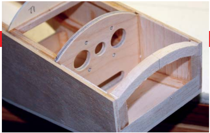
This shows a front view of the fuselage before the 1/8-inch balsa front and 1/8-inch balsa top sheeting have been installed. The upper curved piece of 3/8-inch balsa has the back sanded off so that its cross-section is triangular (refer to the side view on the plans). Also visible are the lower 3/4-inch triangular piece and the 3/8-inch triangular pieces on the left and right sides.
