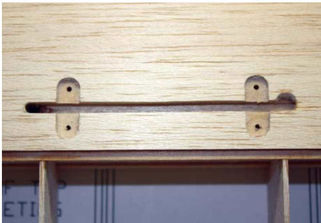
The lower D-tube sheeting has been removed above the slot in the landing gear mount. A little extra sheeting was removed at the outer end of the slot to accommodate the forward sweep and torsional movement of the landing gear. The 1/16-inch diameter screw holes have been drilled for the landing gear strap.
