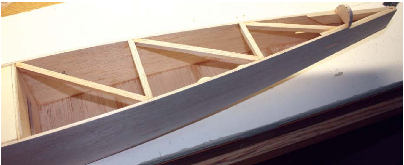
This is a top view of the fuselage before turtledeck formers T6 and T7 and the stringers have been added. Crosspieces at the T6 and T7 positions, turtledeck former T8, diagonal braces, and the stabilizer doublers are shown. Barely visible are the edges of the two cooling-air exit holes in the bottom fuselage sheeting.
