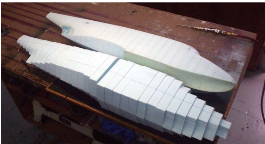
Before and after: This method greatly reduces the time required to shape the fuselage and increases accuracy. Because you only sand off the corners of the sections, it is surprisingly quick.
