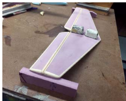
The horizontal stabilizer is shaped using sanding guards at the root and tip because the surface is so thin. The hinge line and edges have balsa bonded to them for protection and additional strength before the 1/2-ounce fiberglass cloth is applied.
