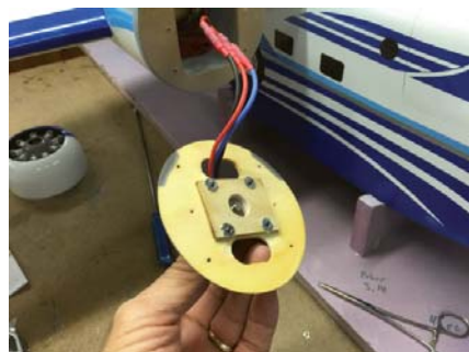
The firewall is made up of three light plywood parts that provide motor and cowl support as well as access for ESC servicing. Assembly is done with internal hex-head wood screws through the cowl.
