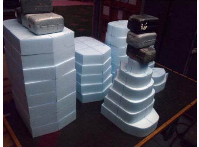
The sections are tack-bonded together to prepare the fuselage for shape sanding. It is best to only manage a few bonds at one time to be sure the centerlines and waterlines stay aligned.
