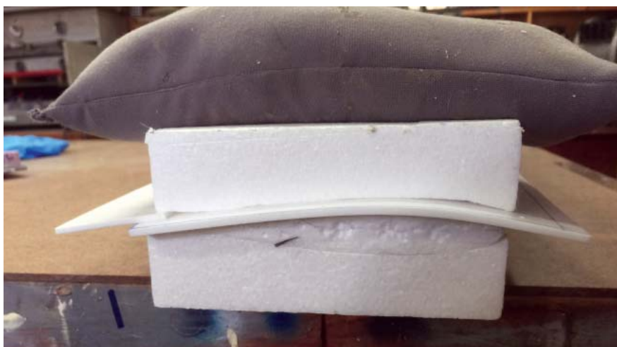
Gorilla Glue is used to bond the foam sheeting to the foam core. Sandbags and the foam bed are used to apply pressure evenly for a complete bond. The drying time is overnight.
