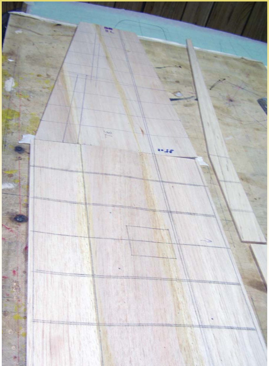
The bottom skin panels are temporarily held together with masking tape. The location of the main spar and the ribs is transferred from the drawing to the bottom skins.
