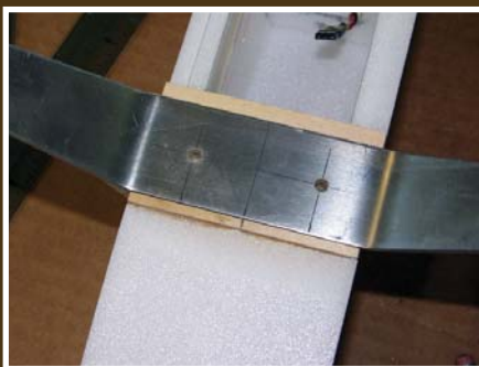
Drill and tap the landing gear plate for #10-24 nylon screws.
