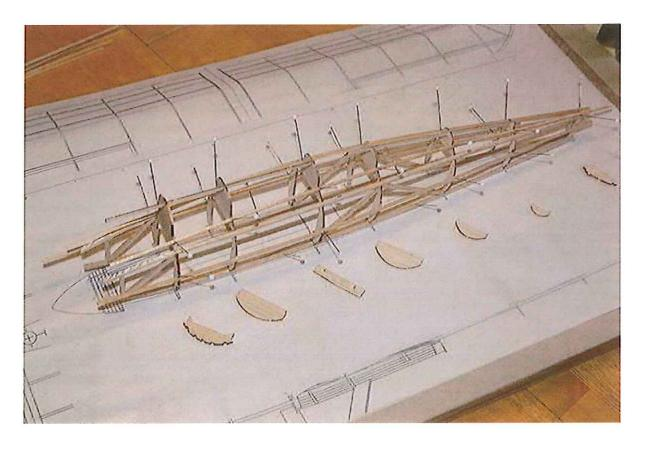
Side frames are joined with upper formers, keels, and a stringer on each side. The bottom formers go in next.
