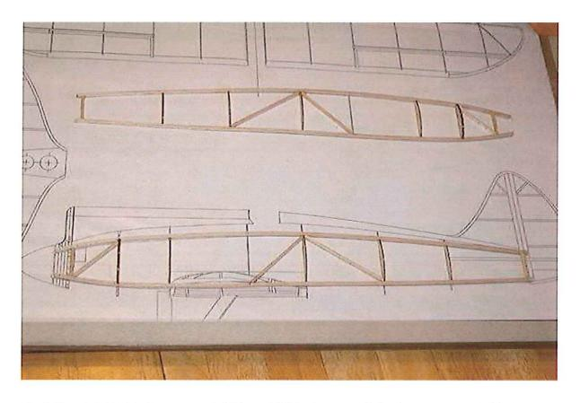
The left and right side frames are built from 3/32-inch square balsa longerons and side formers.
