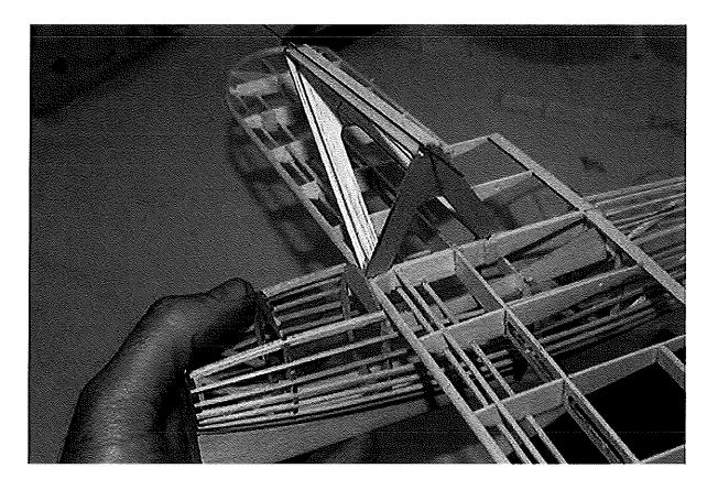
The center ribs are reinforced with scrap balsa to accept the Pete's spindly landing gear. Bracing wires running out to the wings provide needed support.
