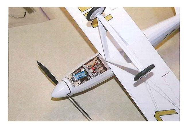
The Pete's internals and unique landing gear arrangement can be seen to good effect.
