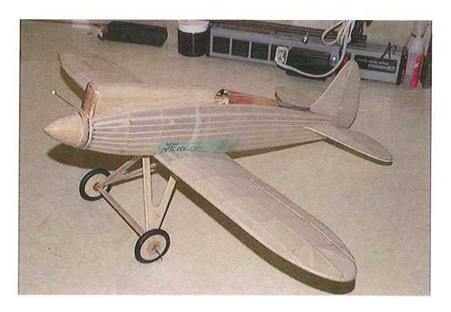
The Pete is covered in tissue, sealed with water-based polyurethane, and is ready for the paint shop.
