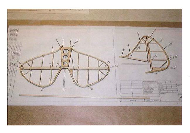
Laminated outlines, kit parts, and 1/16 x 3/32-inch bracing make up the lightweight tail group.
