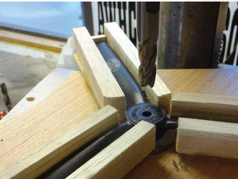
The front of the propeller was drilled to 7/16 diameter, at a depth of 1/8 inch. This is necessary to completely tighten the propeller. The fixture to hold the propeller was built from scrap wood.
