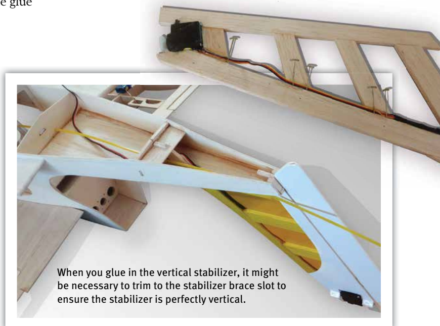
The elevator servo is epoxied to the vertical stabilizer. The servo's front mounting tab has been cut off.
